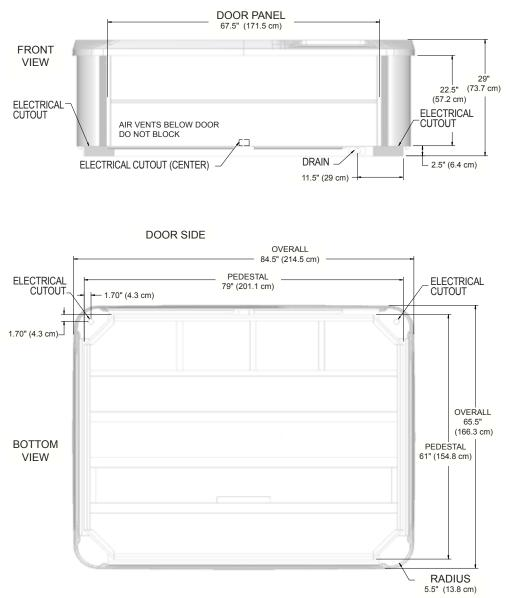
**NOTE: WATKINS WELLNESS** recommends that the STRIDE be installed on a minimum 4" (10.2 cm) thick reinforced concrete pad or structurally sound deck able to support the "dead weight" found in the spa specification chart.
