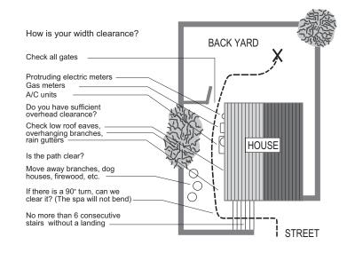
If the spa has to be taken off of the cart to go over a wall (either because the entry area is too narrow, the eaves are too low, the corner is too tight, or the stairway is too steep), a crane will be required. Don't be alarmed! About ten percent of the time, a crane is the only way to install the spa by lifting it to its final destination.
