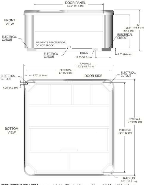
NOTE: WATKINS WELLNESS recommends that the SX be installed on a minimum 4" (10.2 cm) thick reinforced concrete pad or structurally sound deck able to support the "dead weight" found in the spa specification chart. IMPORTANT: THE SX MUST NOT BE SHIMMED IN ANY MANNER.
