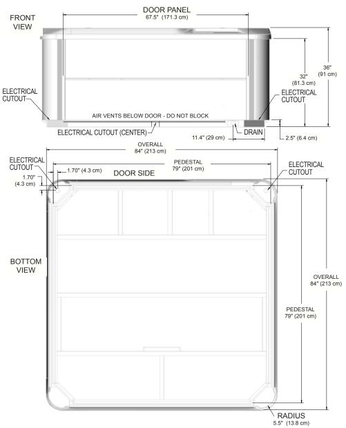
**NOTE: WATKINS WELLNESS** recommends that the Relay & Rhythm be installed on a minimum 4" (10.2 cm) thick reinforced concrete pad or structurally sound deck able to support the "dead weight" found in the spa specification chart. **IMPORTANT:** THE RELAY & RHYTHM MUST NOT BE SHIMMED IN ANY MANNER.
