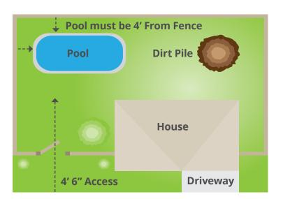
The installation crew will require the location of the plumbing equipment for the purpose of where to orient the **skimmer and return cut out.** These are pre-cut in the pool walls so once the wall has been erected this location will be unable to be changed.
